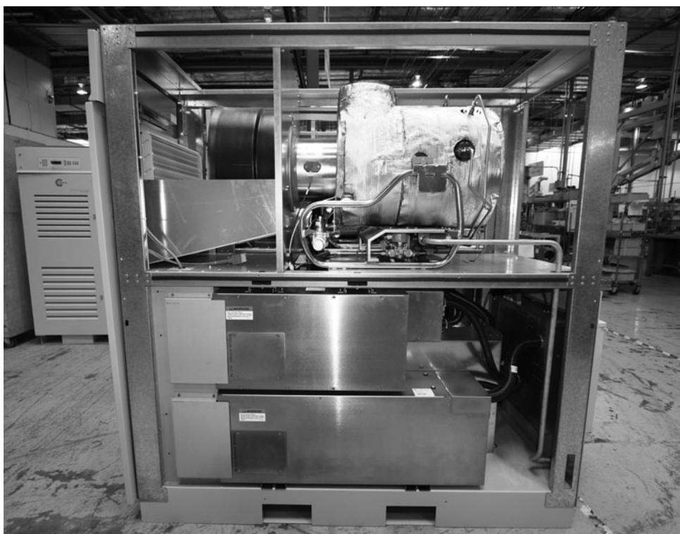
**Figure 12.7** A microturbine assembly. *Courtesy of Capstone Microturbine.*
