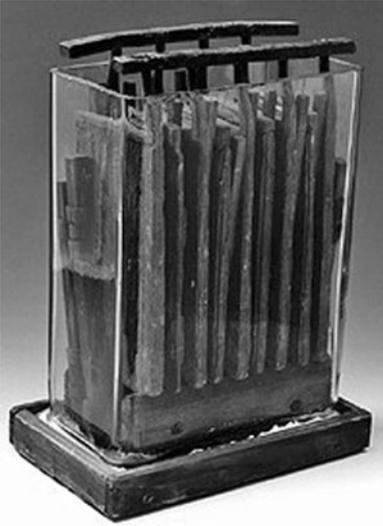
**Figure 3.40** Alessandro Volta's pile.
