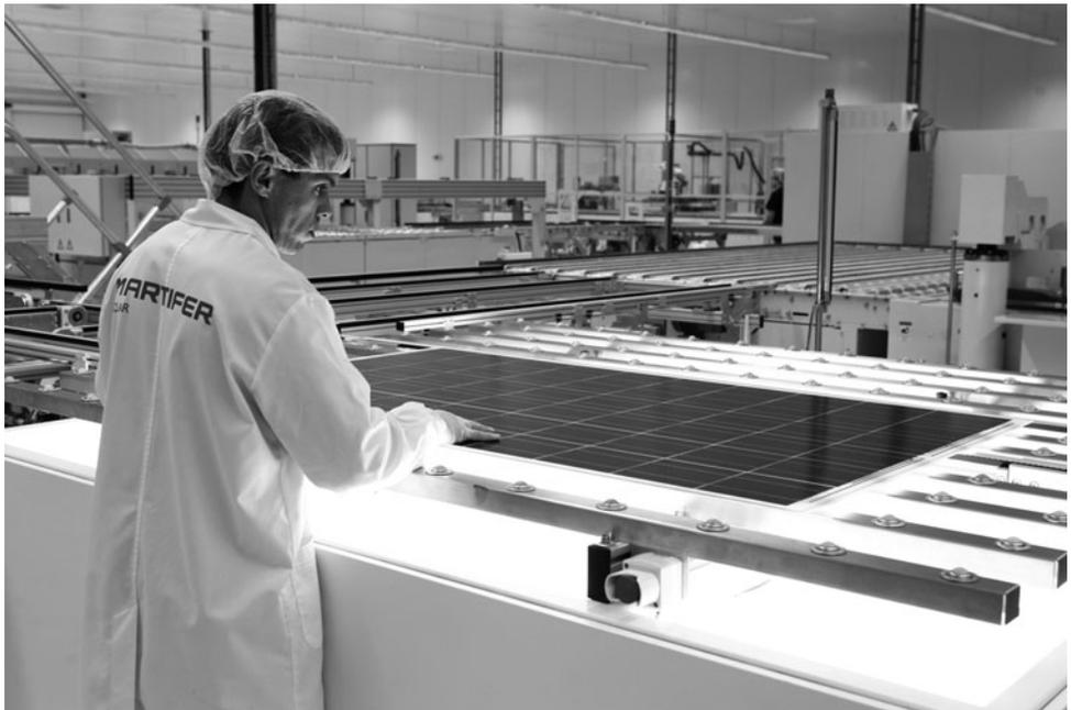
**Figure 3.20** A solar panel inspection station. *Photo courtesy of MARTIFER.*
